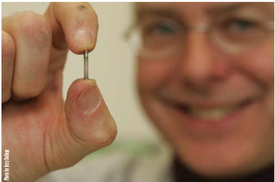
**Small wonder**—VA prosthetics engineer Dr. Richard Weir displays an implantable myoelectric sensor. The devices, now in development, would be injected into muscles and pick up electrical signals to drive artificial limbs. Read more about Weir’s leading-edge work inside.
